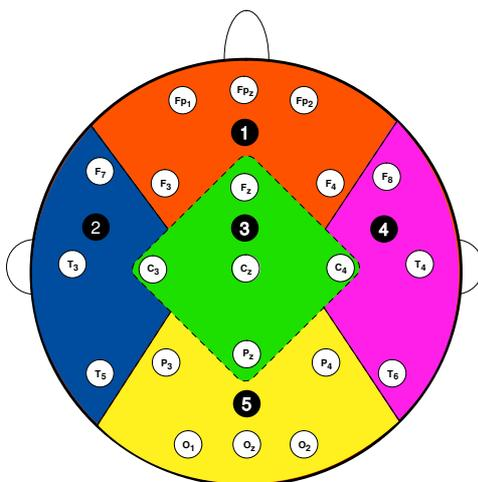
Fig. 5. The 21 electrodes used for EEG recording, distributed according to the 10–20 international placement system (18). The clustering into  $N_R = 5$  zones is indicated by the colors and dashed lines (1 = frontal, 2 = left temporal, 3 = central, 4 = right temporal and 5 = occipital).
