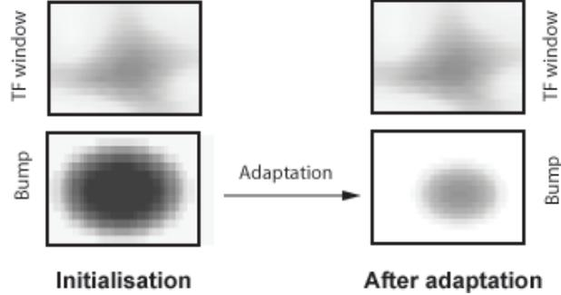
Fig. 4. Learning the bump parameters by minimizing the quadratic cost function (49); Top (left and right): a given patch of the time-frequency map. Bottom left: initial bump; Bottom right: bump obtained after adaptation.
